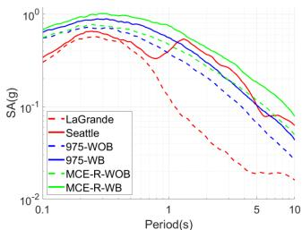
Figure 2: Average response spectra of ground motion suites considered in the assessment, including simulated M9 (Seattle and LaGrande), and ground motion shaking (with -WB- and without -WOB- basin effects) consistent with a 975-year return period and MCE-R shaking.
