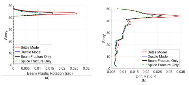
Figure 5: Median (a) plastic rotation of the beams and (b) story drift ratio results of Seattle M9 simulations for structural models with and without beam-to-column and column splice fracture-prone welded connections.
