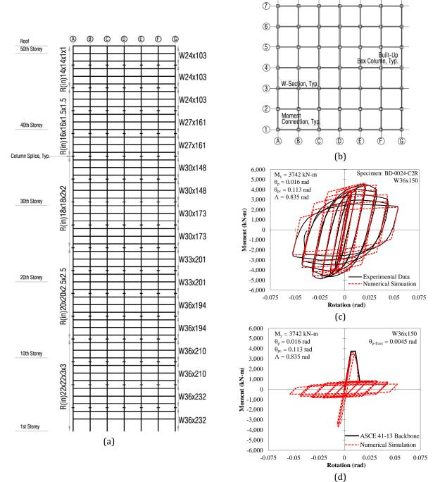
Figure 1: Archetype steel moment-frame building (a) elevation, (b) plan, and sample hysteretic responses of (c) ductile vs (d) fracture-prone beam-to-column connections. Adapted from [8].
