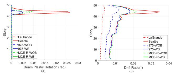
Figure 4: Median (a) plastic rotation of the beams and (b) story drift ratio results of ground motion suites considered in the assessment, including simulated M9 (Seattle and LaGrande), and ground motion shaking (with -WB- and without -WOB-basin effects) consistent with a 975-year return period and MCE-R shaking.
